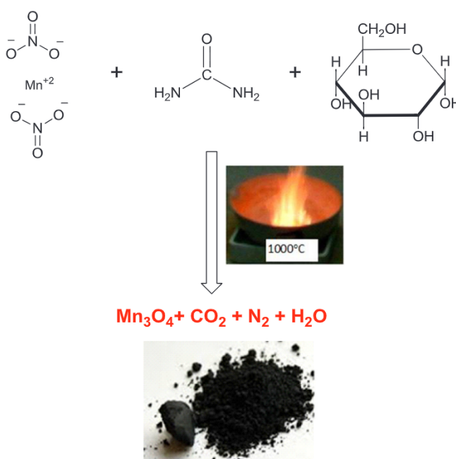
Fig. 2. Steps of the chemical reaction of combustion method.
